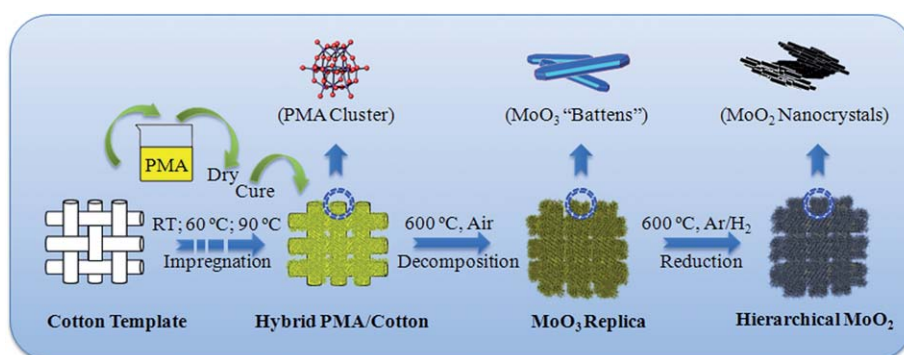
Scheme 1 Schematic illustration of hierarchical \text{MoO}_2 formation.
